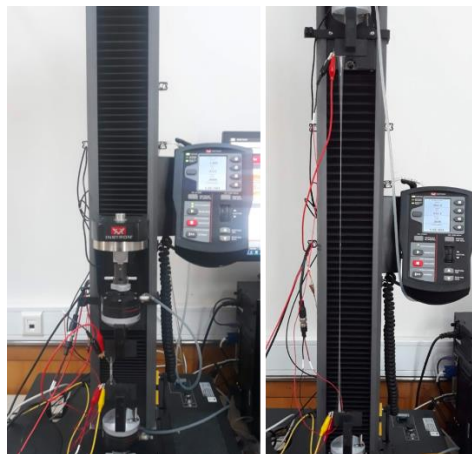
Supplementary Figure 17. Strain test setup. An example of a sample at 0%, and ~900% strain.
