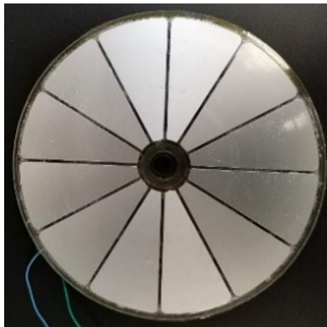
Supplementary Fig. 18 Device abrasion photographs of stator of S-TENG after 100 thousand times cycles.
