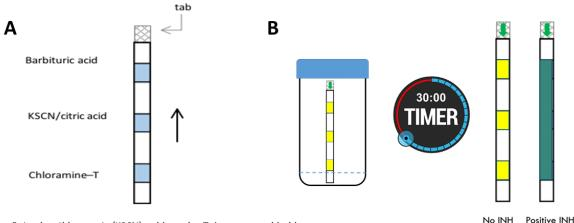
♦ Potassium thiocyanate (KSCN) + chloramine T  $\rightarrow$  cyanogen chloride
