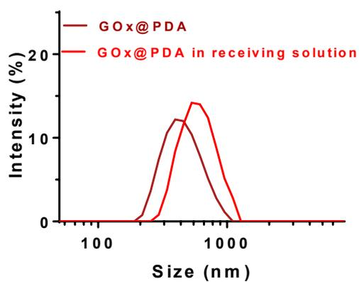
**Figure S18.** DLS measuring the size of GOx@PDA before and after penetration into skin.
