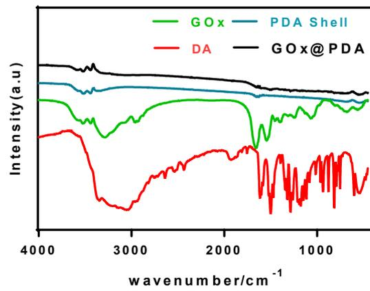
**Figure S3.** FT-IR spectra of GOx, DA, PDA shell and GOx@PDA.
