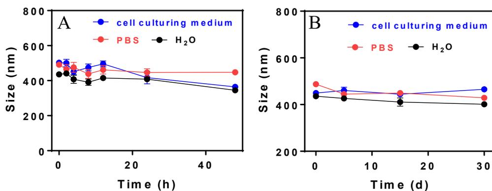
**Figure S5.** (A) Dynamic particle size change of GOx@PDA in water, PBS (pH 7.4), and cell culturing medium at 37 ° C for 48 h incubation. (B) The long-term colloidal stability of GOx@PDA at 4 ° C.
