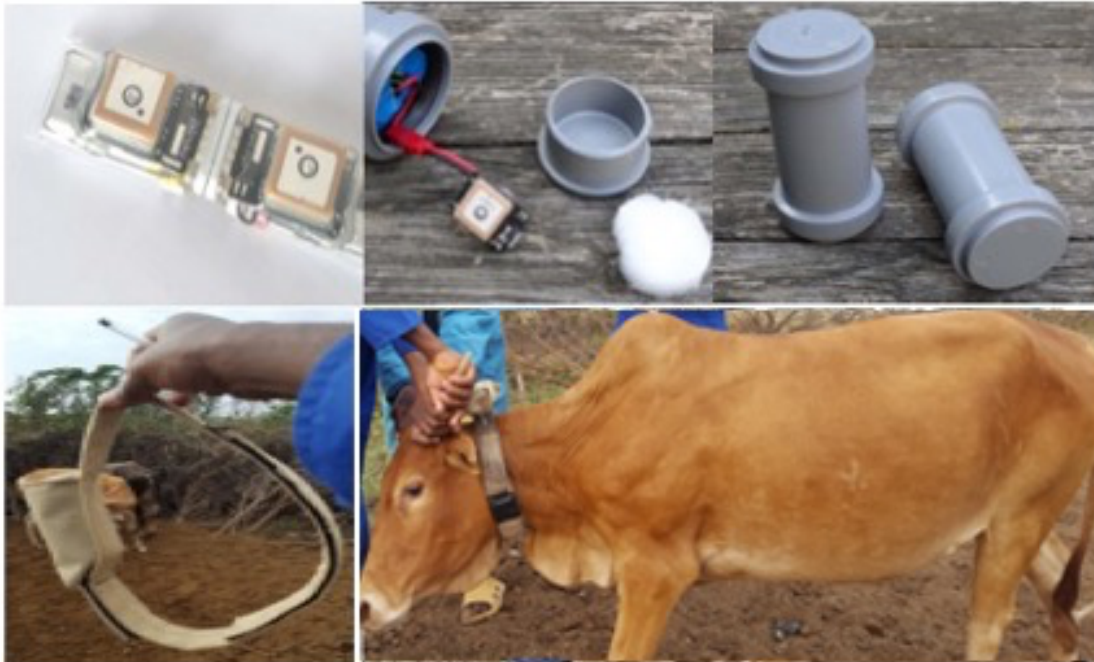
Figure S1. Pictures showing the components of Global Positioning System collars used in the study to track movements of individual cattle in a herd. Complete units were mounted on cattle using locally-produced collars.
