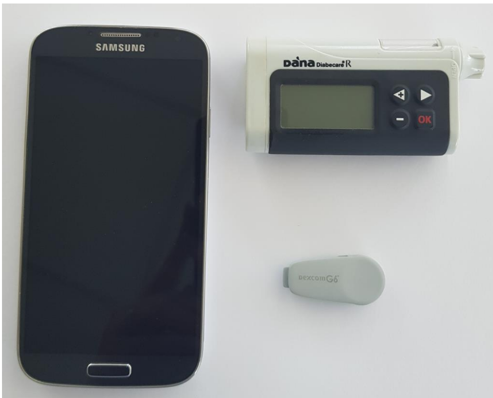
Figure 1: CamAPS HX comprises Samsung Galaxy phone (or similar) running Cambridge control algorithm, Dana insulin pump (Sooil), G6 real-time CGM sensor (Dexcom).
