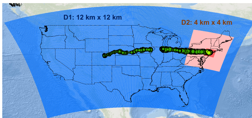
Fig. S12. The continental US (CONUS) is modeled at 12 km x 12 km resolution, which feeds a nested Eastern US domain at 4 km x 4 km resolution. The dark pink area denotes the New York City region where we calculate model-observation statistics of surface ozone. The mobile van drive track across the US (green circles, sized by isoprene mixing ratios) are used to assess biogenic emission inventories.
