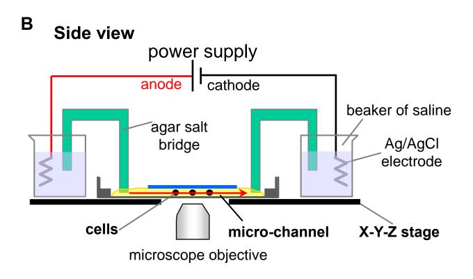
**sFigure 2 Experimental design of multi-field chips and field application. (A)** Chip assembled to connect with power supply via a pair of agar bridges. **(B)** Side-on view of field application set up includes DC power supply and Ag/AgCl electrodes isolated from the chip using agar salt bridges.
