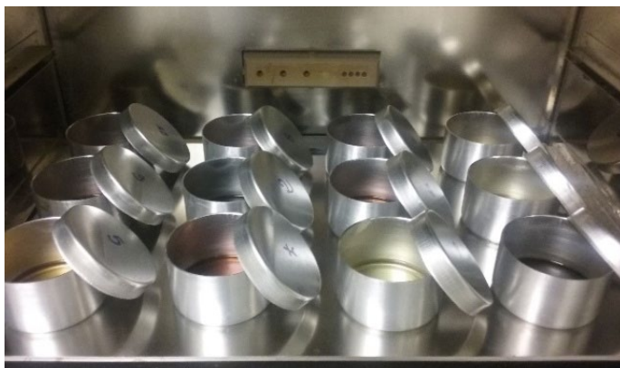
Fig. S4.1. Position of the dishes and lids inside the vacuum oven.
