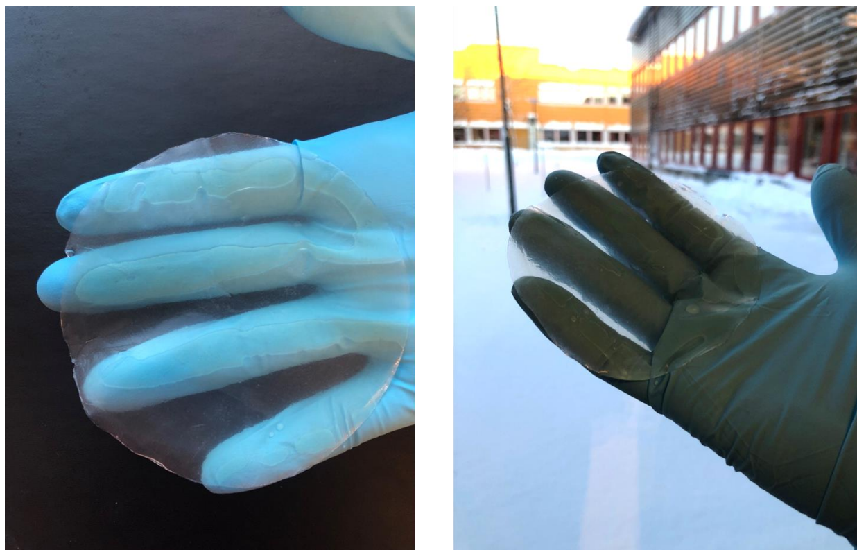
Figure S4. Photographs of the T-GNF hydrogels at 40 \text{ g m}^{-2} after reaching the equilibrium state.
