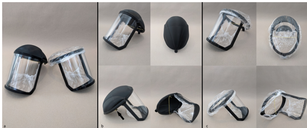
Figure 4 a) Side- by-side comparison of assembled 3D printed helmet with optional top shell (left) or shower cap (right). b) 4 views of assembled helmet with shell. Arrow pointing to boat-cleat attachment-point for elastic. c) 4 views of assembled helmet with shower cap
