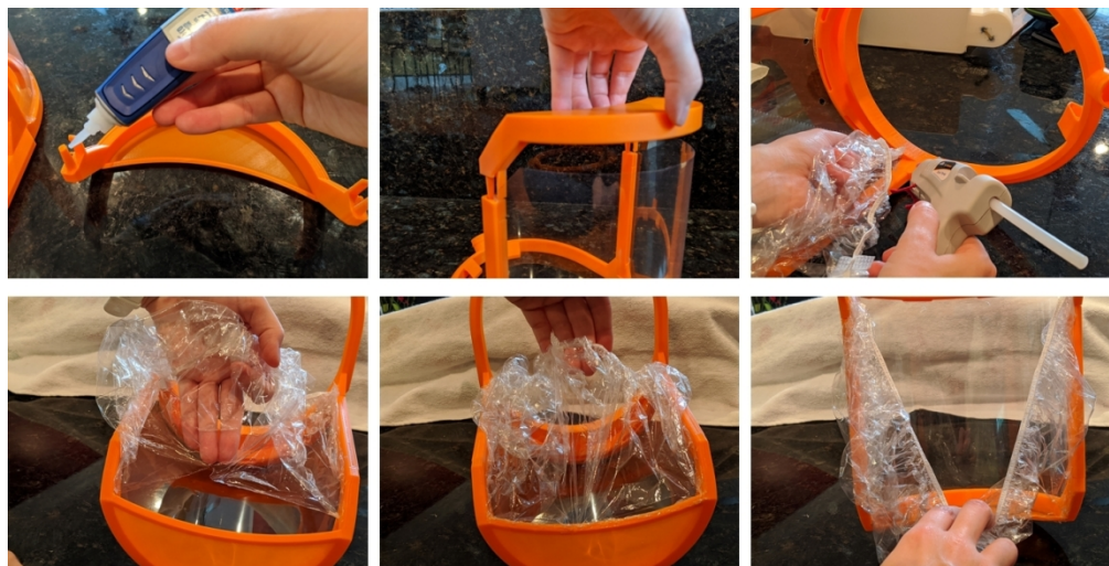
Figure 3 Assembly of jaw piece and application of shower cap. 120x60mm (300 x 300 DPI)
