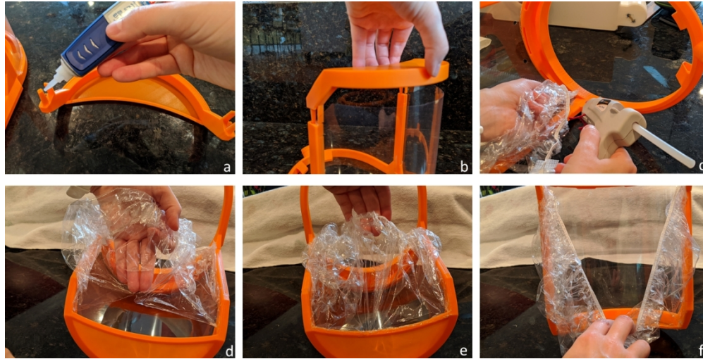
Figure 3 Assembly of jaw piece and application of shower cap. a) Apply CA glue to Jaw Piece joint b) align Jaw Piece and Head Piece with 7 mil cover sheet and join. c) Once shower cap is cut down the center about halfway; hot glue the two sides where the upper jaw piece meets the head piece. d-f) Carefully continue to separate cap down center so that the sides can be hot glued down the side and to the center of the Jaw Piece.
