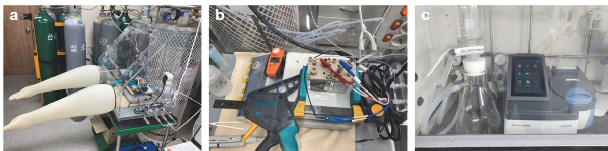
Figure S26. Experimental setup for ensuring safety during the in situ SD quantification with cyanide. (a) Lab-made glovebox filled with Ar gas (which equips gas-inlet/outlet lines), (b) electrochemical cell and other equipment placed in the glove box, and (c) vacuum pump and UV-vis spectrophotometer placed in the fume hood.
