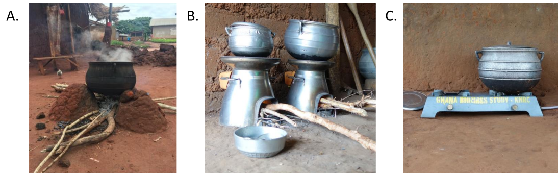
Figure S1. Photographs of representative study cookstoves. Panel A: traditional, open-fire cookstove; panel B: two Improved Biomass (BioLite) cookstoves; and panel C: two-burner liquefied petroleum gas (LPG) cookstove.
