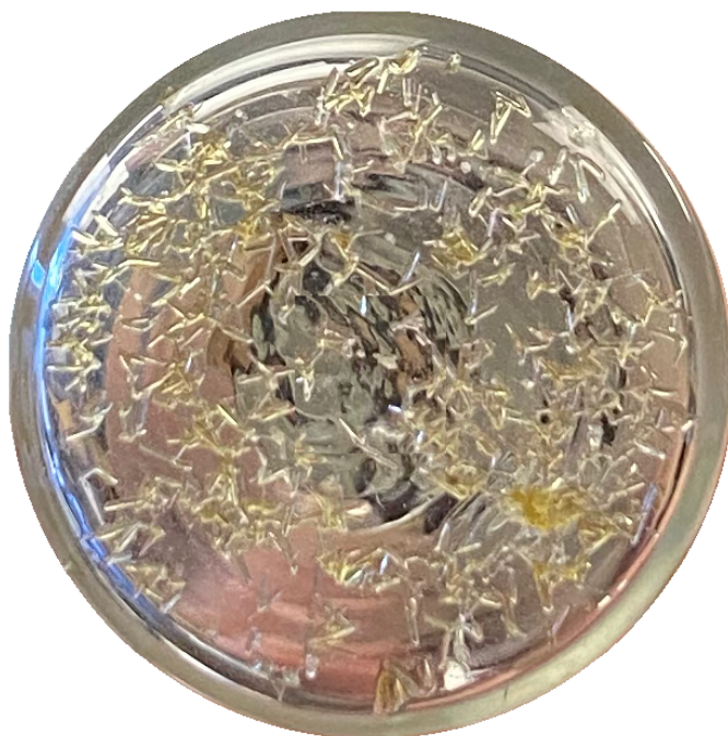
Figure S9. Triketide lactone crystals. After silica gel chromatography, a fraction containing 1 was crystallized in a glass vial.
