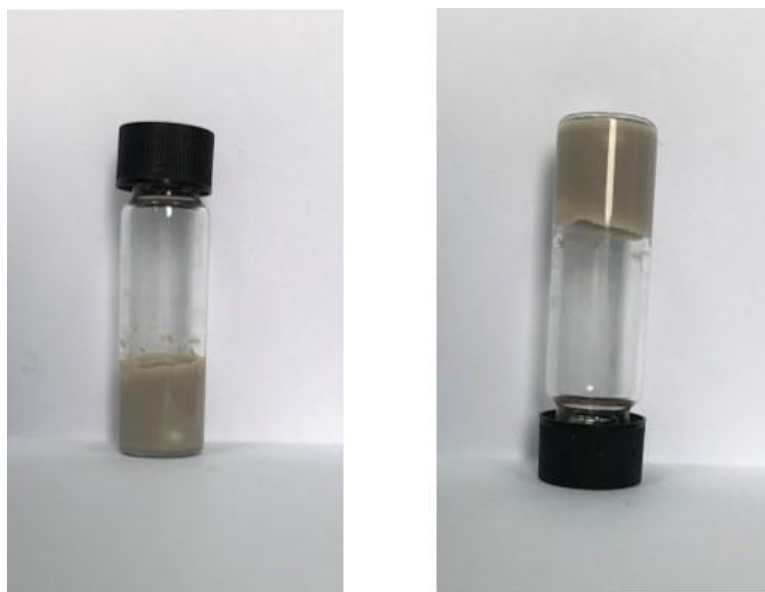
Supplementary Figure 3. The formation of the macro-hydrogel containing \text{Fe}_3\text{O}_4@\text{IHPs} after increasing the feeding amount of AP and Fmoc-Tyr ( \text{H}_2\text{PO}_3 )-OH.
