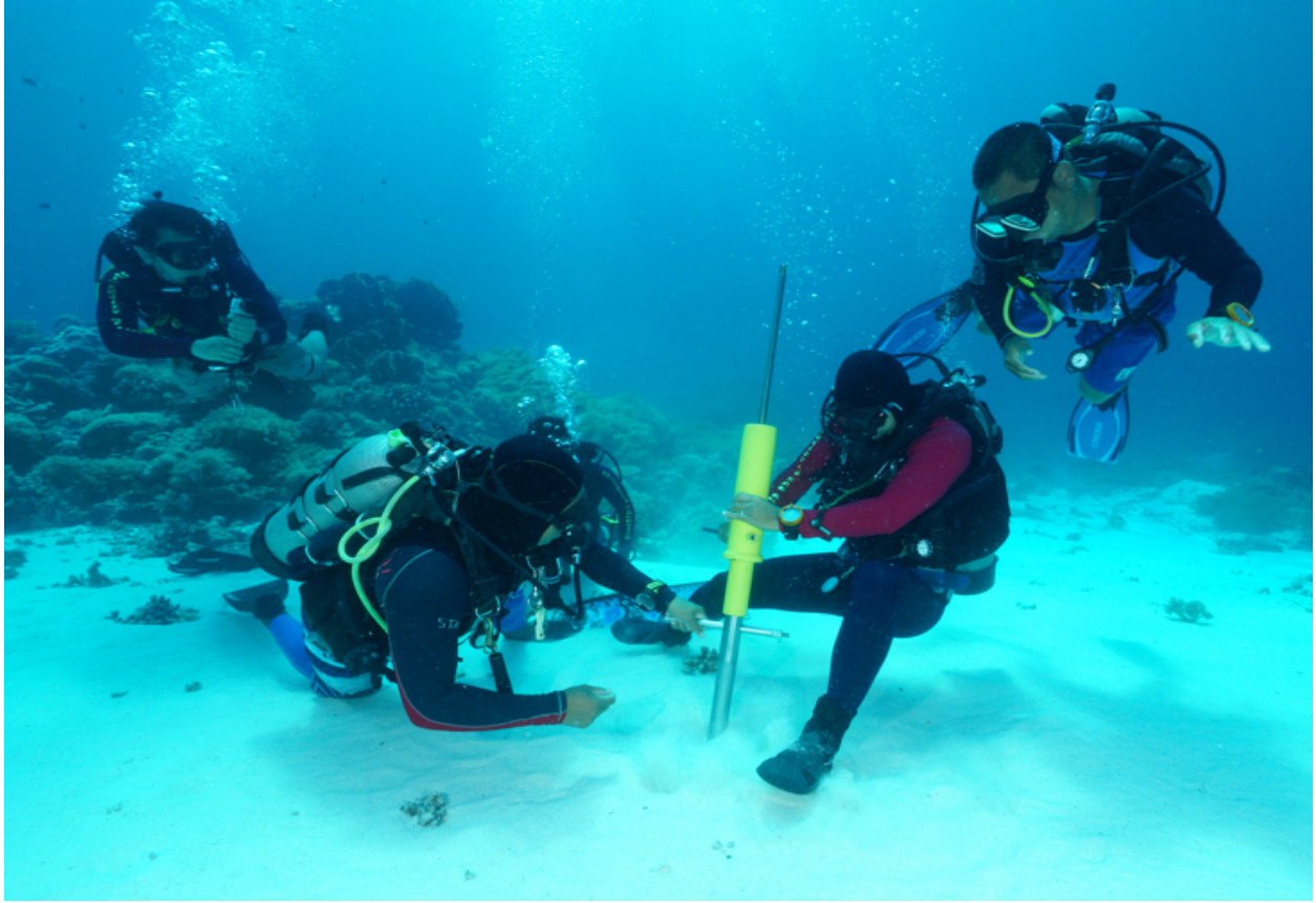
Supplementary Figure S1. Sediment Core Sampling Using a Fabricated 1-Meter Sediment Core Sampler. Marine sediments were collected by manually inserting the piston to the seabed for the core barrel to penetrate through hammering strokes.
