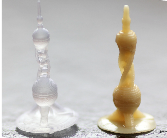
Figure S9. Comparison of Shanghai Oriental Pearl Towers printed by the commercial SLA printer and the smartphone-enabled DLP.
