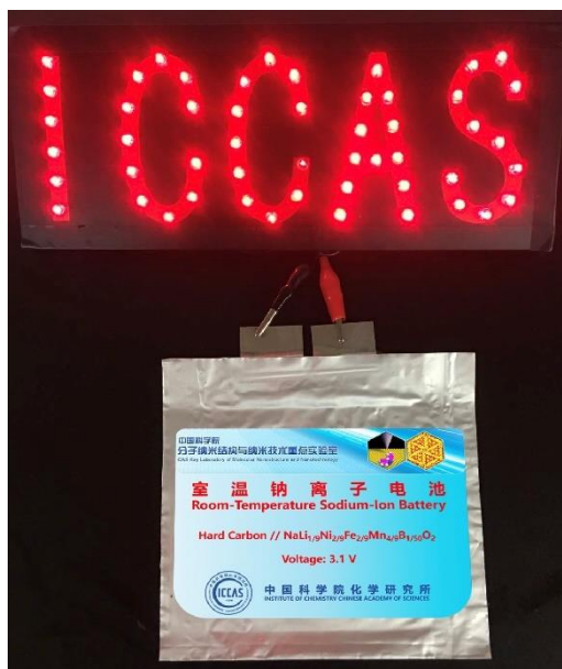
Supplementary Figure 12. Pouch cell of B-doped cathode to power light-emitting diode lamps as proof of concept.
