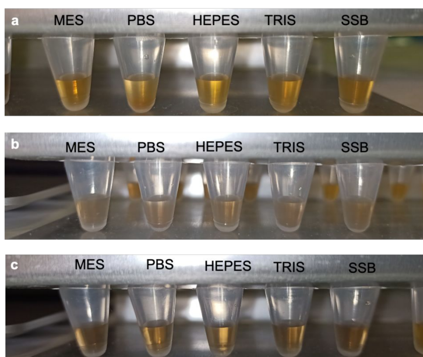
Figure S3. Colloidal stability of CP-DMSA (a), TD-DMSA (b) and OP-PAA (c) samples in different buffer solution: 10 mM MES pH7.0, PBS 1X, 20 mM HEPES pH 8.0, 20 mM TRIS pH 8 and 50 mM SSB pH 9.0.
