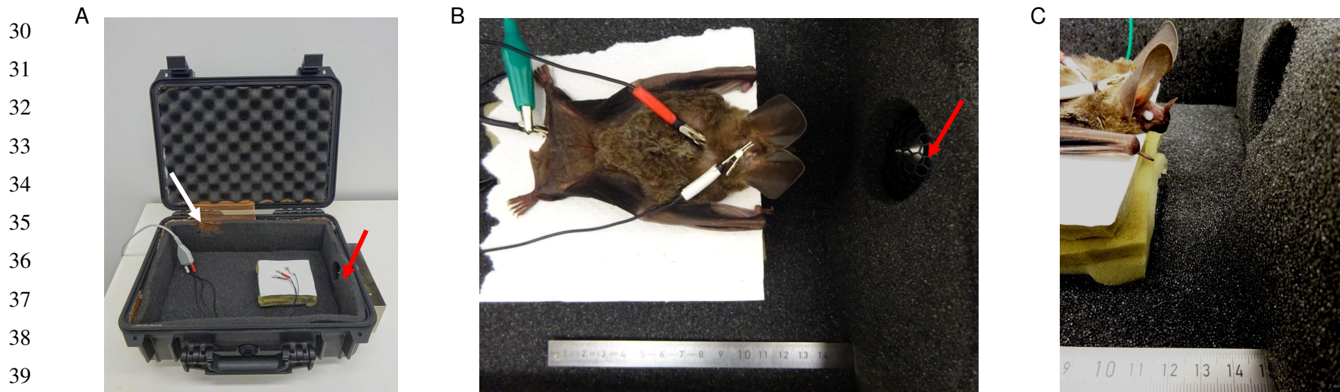
40 Fig. S1: ABR setup and positioning of the individuals. A) Photo of the open small sound-attenuating box, which was electrically insulated with a 41 layer of copper mesh (see part of the mesh between lid and box, indicated by white arrow) and acoustically insulated with sound-attenuation foam. 42 The loudspeaker was embedded in the right side of the box (indicated by red arrow). Small, soft foam pads were positioned in front of the 43 loudspeaker to support the individual and covered with paper towels for hygienic reasons. B) Each individual was carefully positioned facing the 44 center of the speaker (indicated by red arrow) with a 4 cm distance between its outer ear openings and the speaker. To adjust for the different sizes 45 of the individuals, the small, soft, thin foam pads were stacked at different heights. The heads of the bats were always placed at the same level as the 46 center of the speaker. We very diligently checked the head positioning to avoid an off-center angle towards the speaker. The recording electrode 47 (red, plus) was placed at the caudal midline of the head, close to the brainstem and the reference electrode (white, minus) was placed at the dorsal 48 midline of the head between the ears. The ground electrode (black) was placed on the tail membrane, carefully avoiding the calcar. To ground the 49 bat, the ground electrode was connected to the copper mesh of the setup via a crocodile clamp (green). C) Side view: To prevent the bats' eyes from 50 drying, a drop of eye cream was applied. Lophostoma silvicolum is shown as an example.
