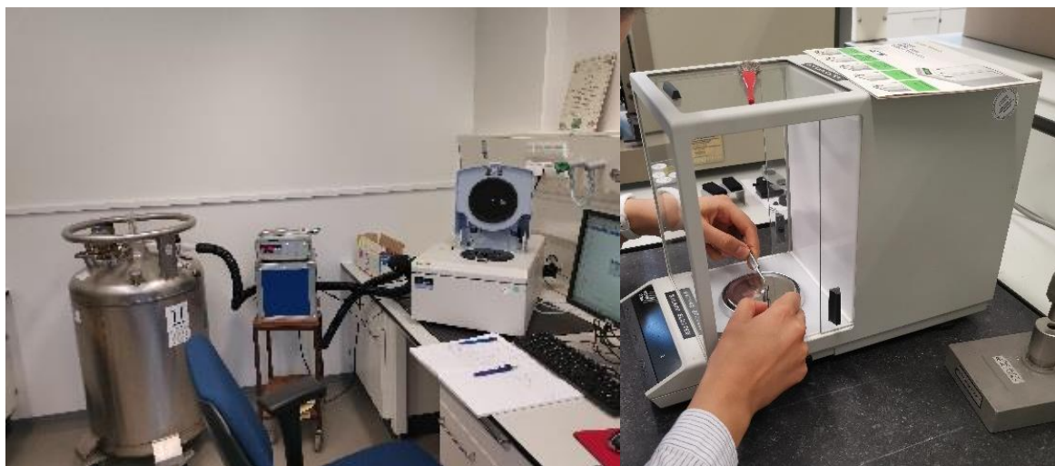
Figure 1. Measurement setups. Left, Differential Scanning Calorimetry (DSC). Right, samples of 5 mg are accurately prepared for XRD measurements.
