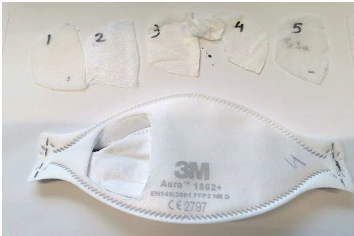
Figure 1. Dissection of 5 constituent layers of 3M Aura 1862+ mask filter.
