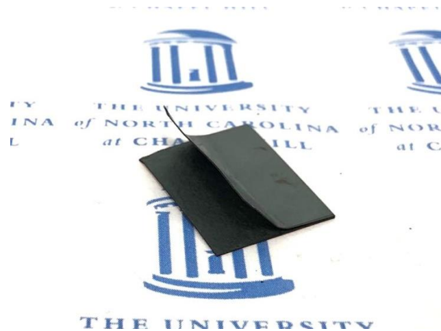
Fig. S2. Photograph of partly peeled-off laminated heterojunction perovskite film. Photo Credit: Ying Zhou, University of North Carolina at Chapel Hill.
