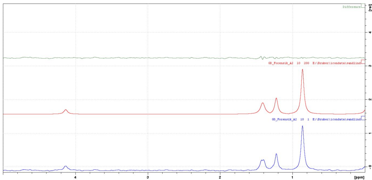
Figure S10. Experimental data of PMP-a2 shown at the bottom (blue), the deconvolution fit shown in the middle (red) and the difference at top (green). The truncations in the deconvolution fit is a graphical error and does not affect the numeric calculations.
