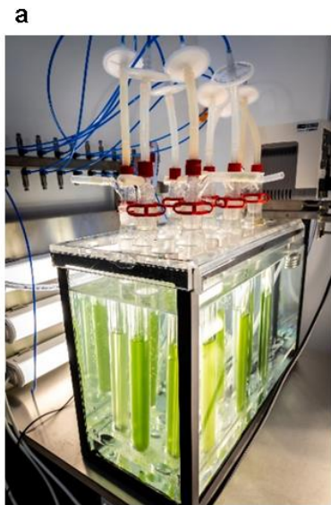
Figure S3. a) Cultivation of Synechocystis in gas washing tubes in an aquarium maintained at 30 °C, air was delivered using a pump and passed through 0.2 µm filters; b) Light intensity measurements for each tube (measured in water).
