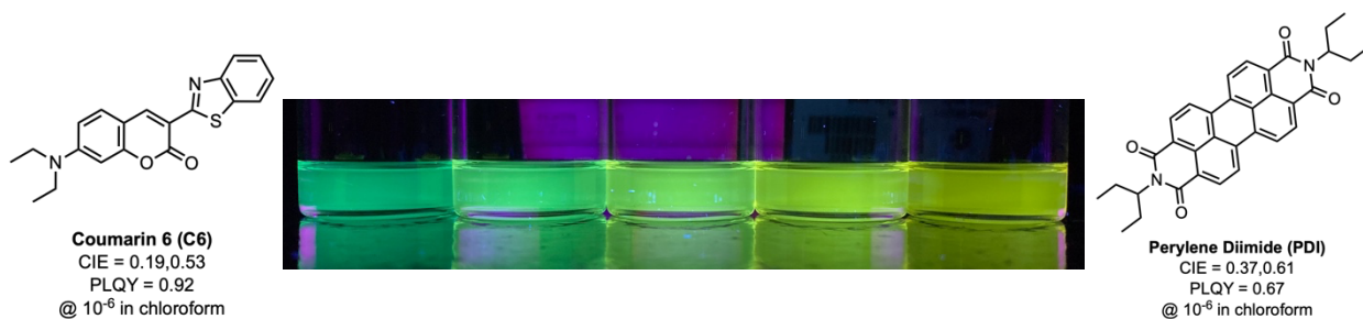
Figure S20. (From left to right) C6 ( 1.2 \times 10^{-6} M), C6: PDI ( 0.9 \times 10^{-6} M: 0.3 \times 10^{-6} M), C6: PDI ( 0.6 \times 10^{-6} M: 0.6 \times 10^{-6} M), C6: PDI ( 0.3 \times 10^{-6} M: 0.9 \times 10^{-6} M), and PDI ( 1.2 \times 10^{-6} M) irradiated with a long wave UV-lamp at 365 nm.
