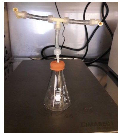
Holding tank setup with T-splitters to flow 58 into multiple lagoons.
