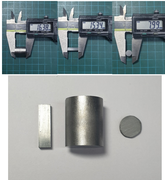
Supplementary Fig. 18. Typical dense pellets obtained by SPS with a diameter of 13 mm and a height of ~16 mm (center) and the specimens cut for measuring electrical (left, a bar with a length of ~15 mm) and thermal transport properties (right, a disk with a diameter of 8 mm) along the pressing direction of SPS. Their relative density is ~96%.
