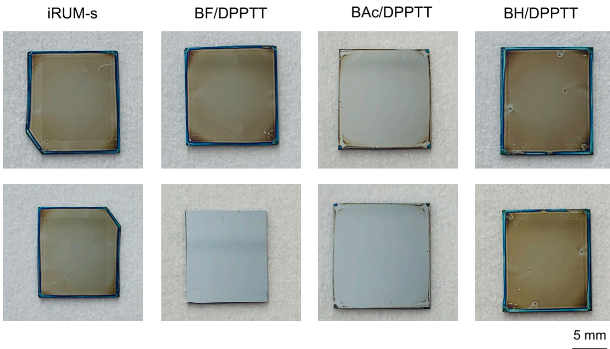
Supplementary Figure 56. Images of iRUM-s film, BF/DPPTT blend film, BAC/DPPTT and BH/DPPTT crosslinked film before (top line) and after (bottom line) soaking in chloroform for 30s.
