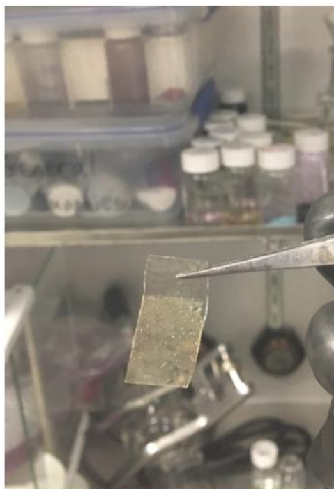
Supplementary Figure 1: Thin film of Mn 3 (C 6 S 6 ) deposited on a glass substrate. Picture on the right is tilted to show thin film interference.
