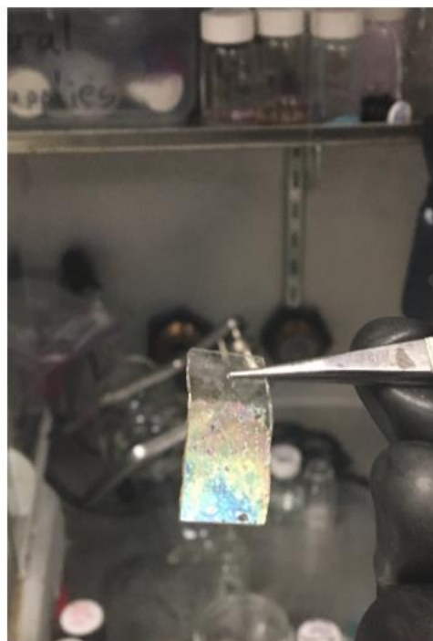
Supplementary Figure 1: Thin film of Mn 3 (C 6 S 6 ) deposited on a glass substrate. Picture on the right is tilted to show thin film interference.
