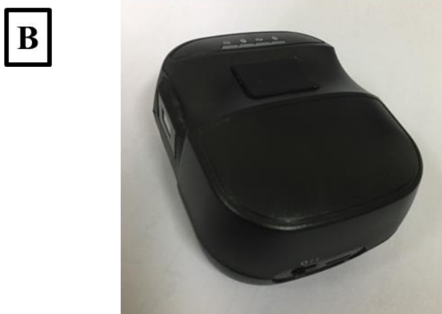
Fig S3 F. Images of the NIR-S-G1 beta version (NIRscan) NIR spectrometer with smartphone used to control the device.
