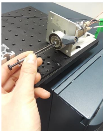
Fig S5.9. Screenshots and images illustrating QDa operation (A) Screenshot of the QDa control window. (B) Screenshot of the sample list window. (C) Image of the six-port injector being loaded by syringe. (D) Screenshot of processing the total ion chromatogram for the API of interest
