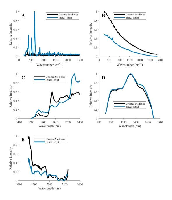
**S22** Appendix. Intact vs. crushed ACA tablet analysis by Raman and NIR spectrometers. Spectral comparisons of a field collected sample of AMK 1000 mg (a co-formulation of amoxicillin and clavulanic acid) are shown with the (A) Progeny, (B) Truscan RM, (C) MicroPHAZIR RX, (D) NIR-S-G1, and (E) Neospectra 2.5 spectrometers. The spectra in blue are scans of an intact tablet of AMK 1000 mg. The spectra in black are scans of the powder from a crushed AMK 1000 mg tablet.
