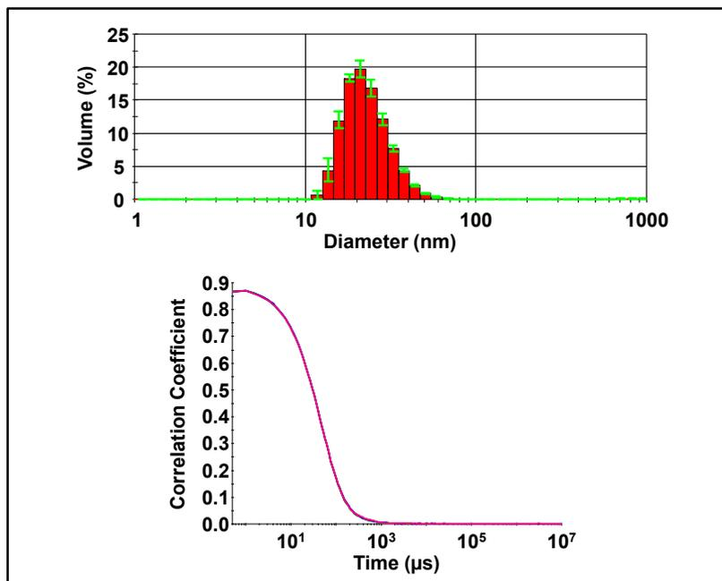
**Figure S3.** DLS histogram and correlation function of PEG-[G1]-DMHCA micelles after freeze-drying and resuspension (10 mM PB, pH 7.4, 150 mM NaCl; 25 °C).
