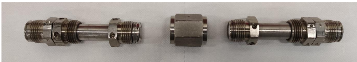
Figure S- 2: Dissassembled flow-through reactors and joint piece
