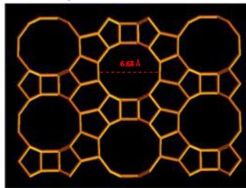
Figure S- 20: Estimation of characeristic dimensions of different lignin oligomers and comparison with β-zeolite pore size
