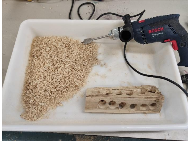
Figure S- 7: Drilling lignocellulose branches to obtain coarse wood sawdust
