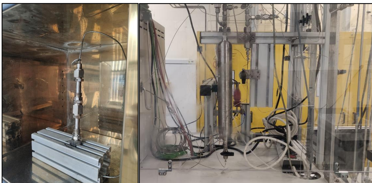
Figure S- 4: a) Assembled reactor in the oven. b) Sample taking section of the setup
