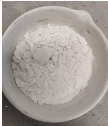
Figure S- 8: Pelletized beta zeolite
