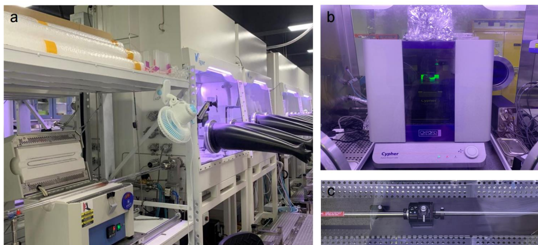
Figure S2. Home built glovebox connected system. (a) Chemical vapor deposition (CVD) tube furnace connected to the glove box. (b) Atomic force microscope (AFM) mounted in glove box. (c) Vacuum transfer holder. The glovebox connected system provides water-oxygen isolation environment for the entire growth, transfer and characterization process of \text{WTe}_2 monolayer to ensure its structural integrity.
