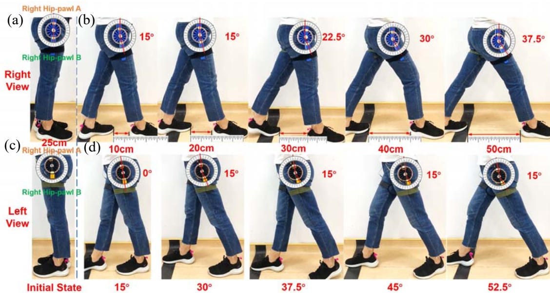
Figure S11. The corresponding screenshot of different step lengths (in the middle of the figure) and angles (at the bottom of the figure) between right and left thigh with two R-TENGs on each hip. (a-b) Right view exhibits the angle between the right leg and vertical axis and the length between left tiptoe and right heel, (c-d) Left view exhibits the angle between the left leg and vertical axis.
