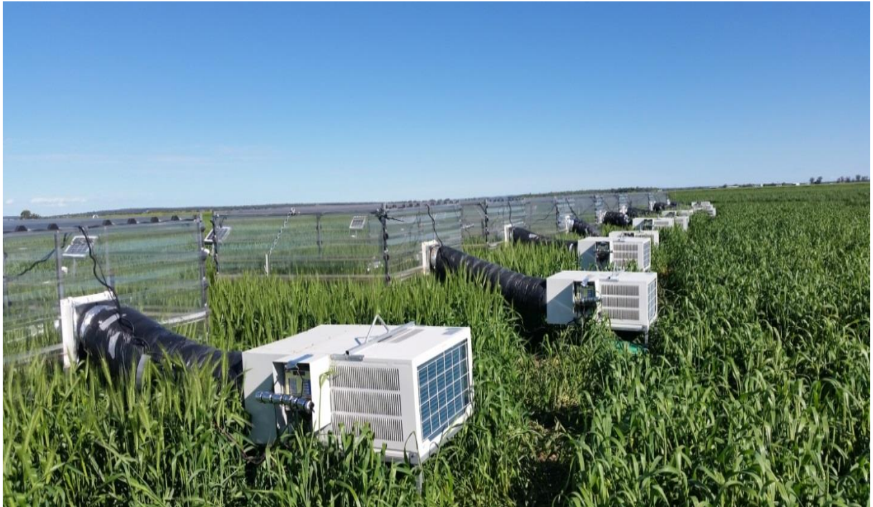
Supplementary Figure 2. Field view of the chambers used to impose heat stress at anthesis during 2016. Set temperatures were achieved using reverse cycle air conditioners (3.9 kW heating and 3.6 kW cooling) powered by heavy voltage generators (15 kVA 3 phase) and controlled using SPLAT (HVAC26A) controllers attached to each unit. Weather-proof temperature and humidity data loggers (HOBO® U23, Pro v2) were used to monitor conditions in each chamber.
