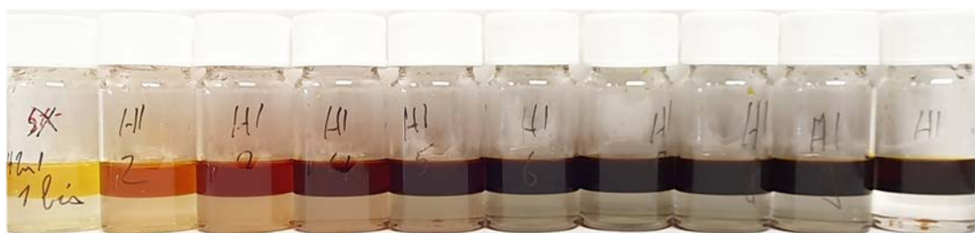
Figure S1. Color evolution of samples containing 0.2 \text{ mol L}^{-1} TOMAI in toluene and aqueous solutions with 0.5 (left) to 5.0 (right) \text{mol}^{-1} HI and \text{ZnI}_2 ( 0.05 \text{ mol L}^{-1} ).
