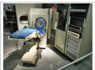
Data General Nova next to EMI Mark I. Left rack contains tape drive. Right rack has the computer and other hardware
