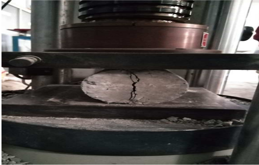
Supplementary Figure 3 Split Tensile Strength Test Setup
