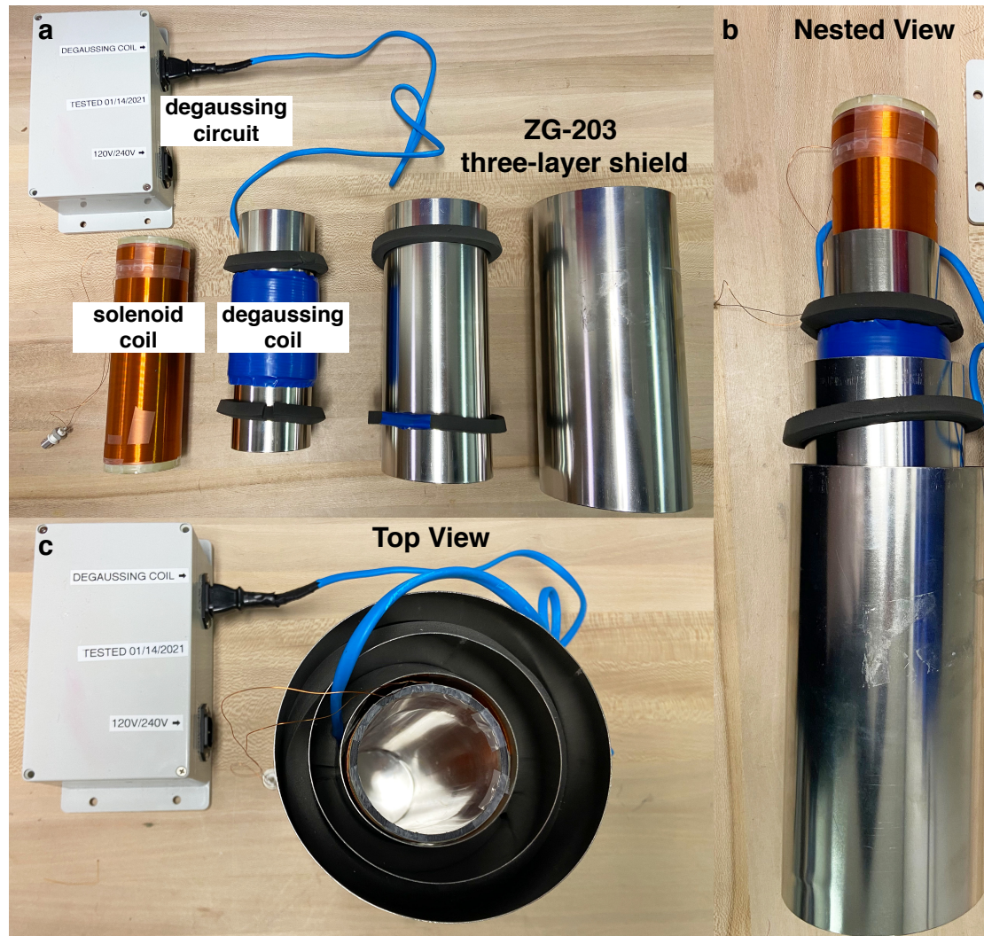
Figure S3. Annotated photographs of three-layer mu-metal shield (Magnetic Shield Corp., P/N ZG-203) equipped with vendor's with degaussing coil: a) view of the disassembled setup showing the connection of the degaussing coil to the degaussing circuit in the electric enclosure; b) nested view of the partially assembled me-metal shield equipped with degaussing (blue) and RF solenoid (dark amber) coils; c) top view of the assembled setup;
