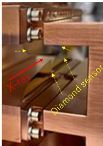
Figure S3 Frontend XBPM-1 with the four-quarant thin diamond pieces (dotted arrows) fixed on copper cooling blocks.
