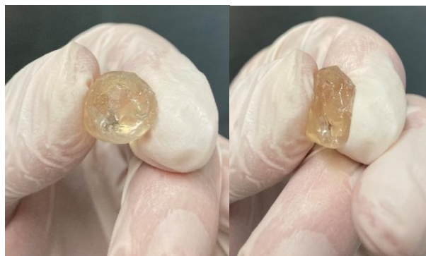
Figure S17. Pictures of the polyCOE obtained from the reaction of COE (1.0 equiv.) with 10 ppm of Ru8 in neat with light activation.
