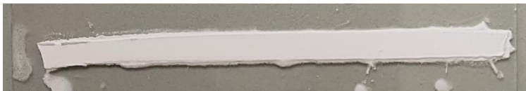
Figure S6. Adjustment of the solids contents of the pastes with HefCel (Ca-H and CaP-H) did not improve printability due to poor water retention.
