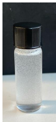
Figure S7: Picture illustrating a styrene droplet in deionized water + Pluronic F108 (0.86 mM). Phase separation was observe after 2 hours and no latex was formed upon shaking.
