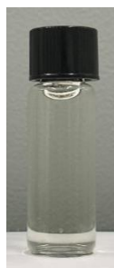
Figure S10: Digital photo of an aqueous solution of SDS (0.25 mg of SDS in 2 mL of deionized water) and macro-CTA (25 mg) with styrene (35 \mu L) on the top (without shaking).
