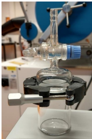
Figure S2. Image of a glass-reactor used in the gas-phase ethylene pre-polymerization of the metallocene-based catalyst materials.
