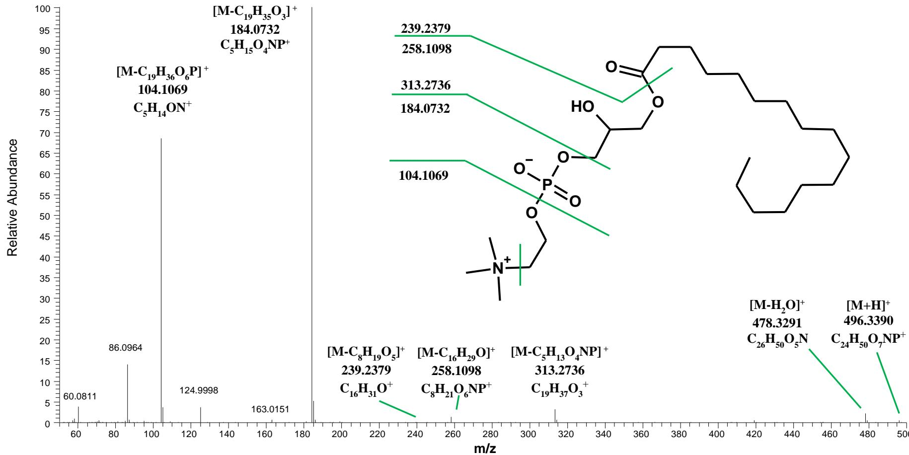
The analogous LysoPC (16:0, 0:0) MS/MS spectrum in a pooled R<sup>+</sup>/R<sup>-</sup> sample. The phosphocholine fragment ions dominate, the acyl moiety shows similar features as those observed in the MGTA (16:0, 0:0) MS/MS spectrum (I). For reference, e.g., refer to Metlin database, ID 182.
