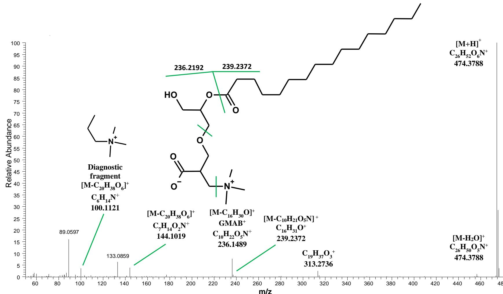
The MS/MS spectrum of the **MGTA (C16:0, 0:0)** in a pooled P+/P- sample. The GMAB diagnostic ions at the lower end of the spectrum, in particular  $m/z$  100.1121 and 144.1019 prove the structure of the N,N,N-trimethylalanine headgroup. A loss of the hexadecyl acylium ion ( $m/z$  239.24) show the C16:0 moiety in the monoacyl-betaine lipid structure.
