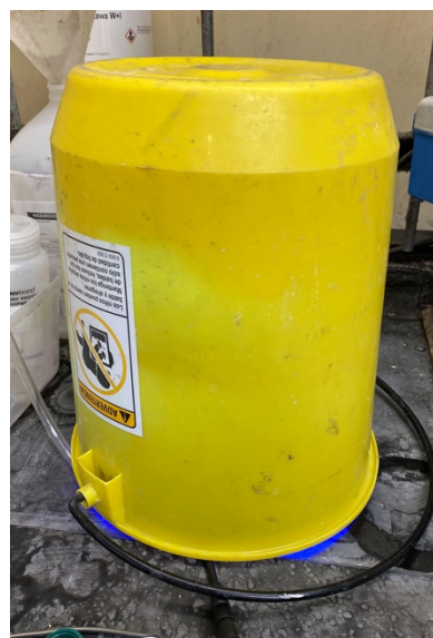
Figure S1. Low-temperature solid-state photoreaction set up for the conversion of 1 to 2a .
