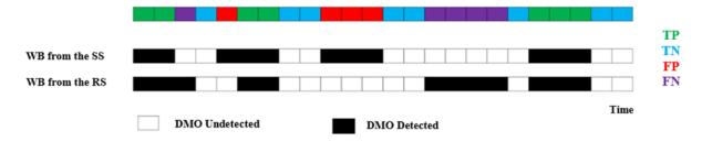
Example of how each sample (0.01 seconds) is identified as TP, TN, FP and FN and compared between the IMU single sensor (SS) and reference system (RS) for the identification/detection of walking bouts. Each sample of the SS and RS outputs are depicted as a rectangle, where white rectangles represent samples of non-WB periods, and black rectangles denote samples of a detected WB period.
